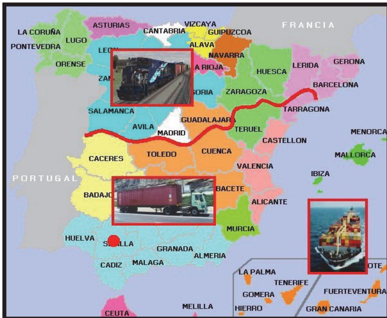
Fig. 16. Cost-effectiveness borders for the different transport modes in Spain for shipments from Seville, as obtained from the decision-making model.
